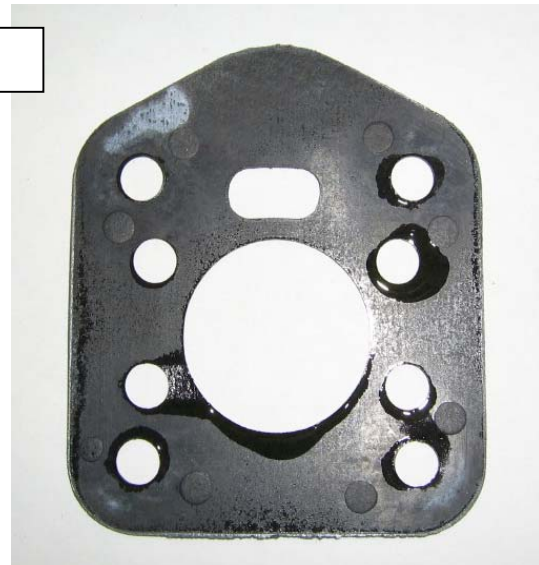
Photo 2- Prop Governor Gasket (Lycoming Shipping Gasket) MUST BE REMOVED
