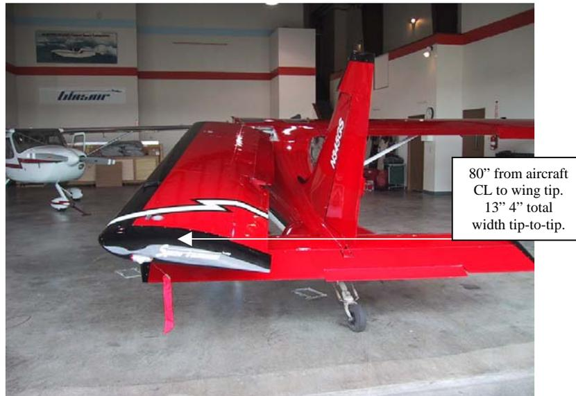
Folding the wings to a tip-to-tip dimension of 13' 4" leaves the flap tracks just outside of fuselage contact. This may be enough to gain optimization of shared hangar space for those not concerned with attaining a road-legal width of 8' 6".
