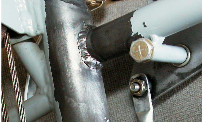
Figure 1. Cracking of weld at tube intersection.
