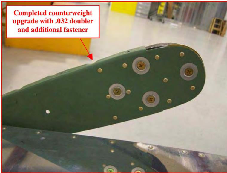
Completed counterweight upgrade with .032 doubler and additional fastener
