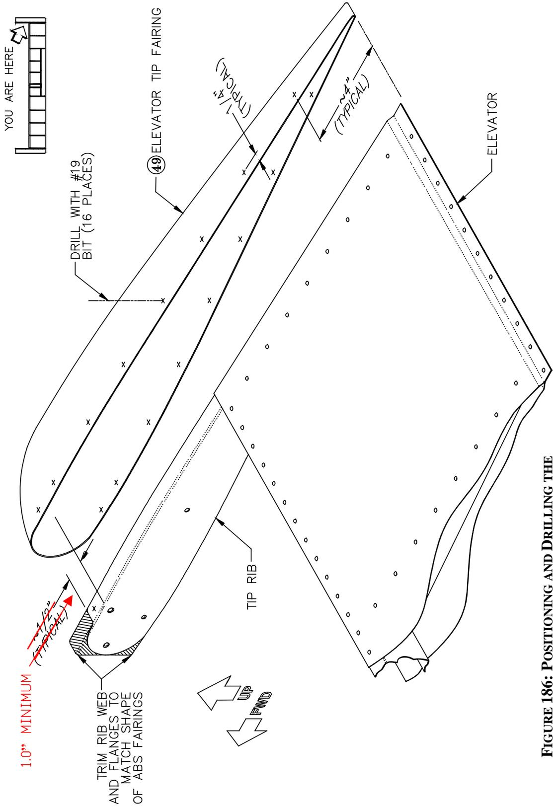
**FIGURE 186: POSITIONING AND DRILLING THE ELEVATOR TIP FAIRINGS**
