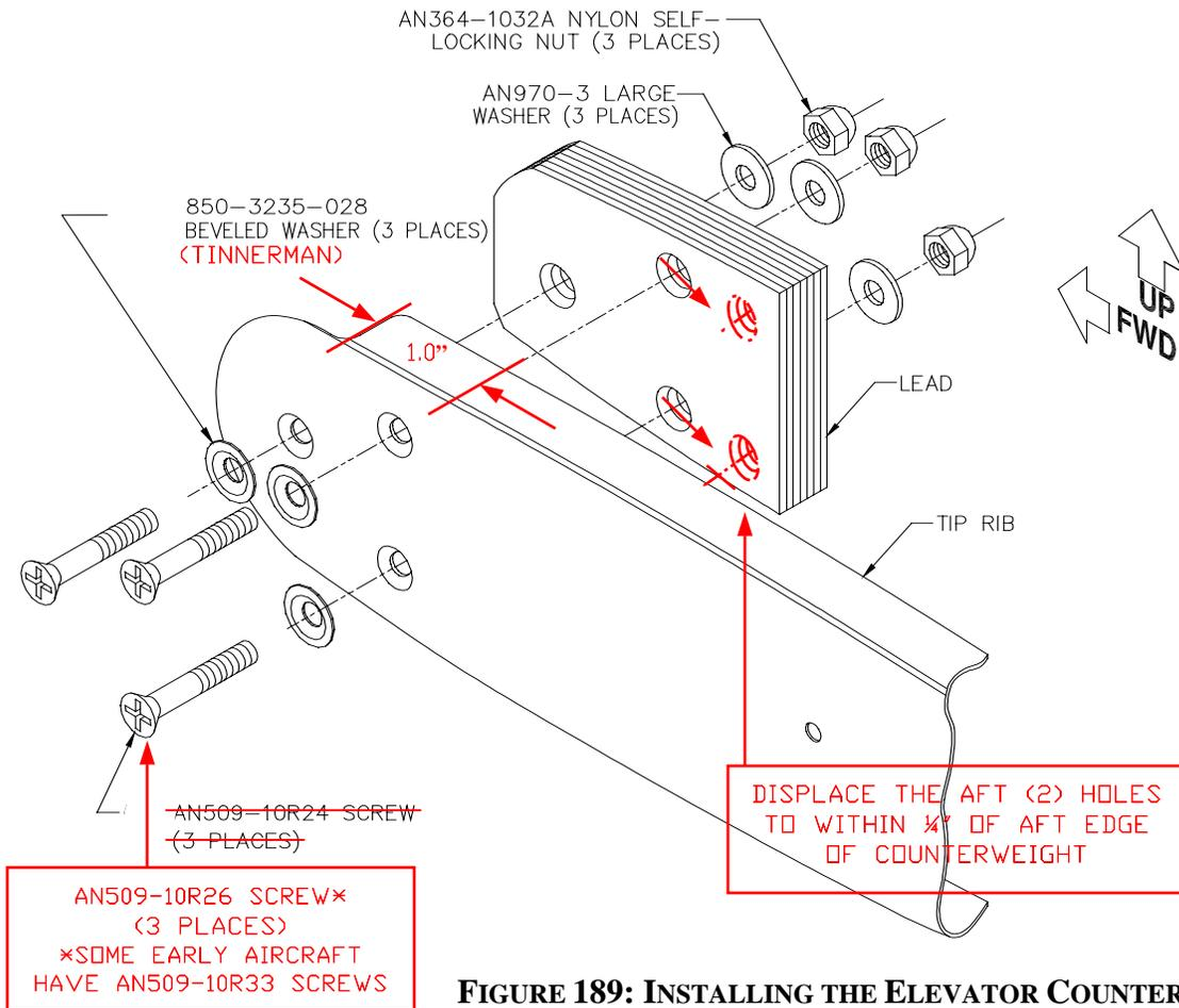
**FIGURE 189: INSTALLING THE ELEVATOR COUNTERWEIGHT**
